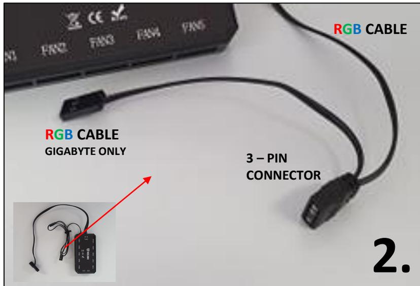
2. Connect RGB Cable from controller to the motherboard.
