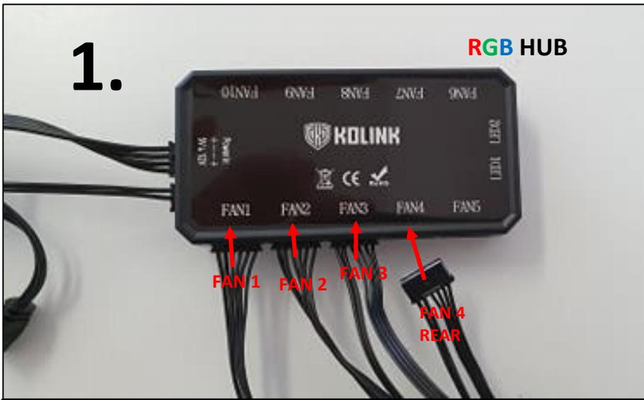
1. Connect fan cables to RGB HUB accordingly. Numbers are visible on the HUB for assistance.
